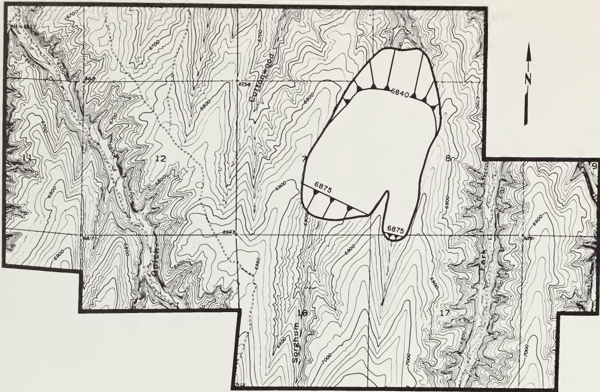
Figure V-16 PROCESSED SHALE PILE: YEAR 5
